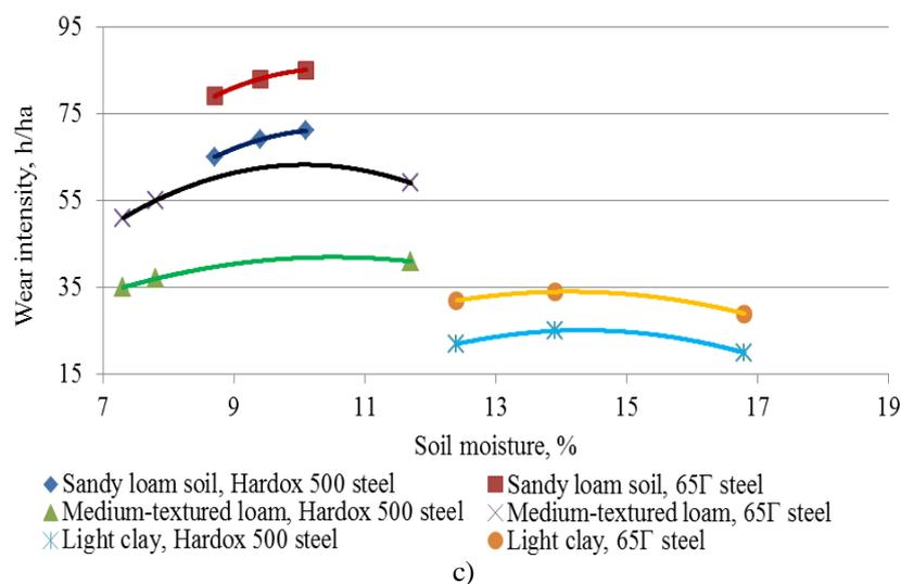
**Fig. 4. Impact of soil moisture on wear intensity of the actuating elements of soil processing machines (experimental data):**
