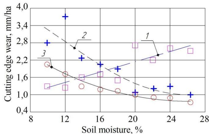
**Fig. 3. Impact of soil moisture on wear intensity of the actuating elements of soil processing machines:**
