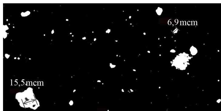
Fig. 1. The size of the particles of titanium-tantalum-tungsten-cobalt hard alloy
