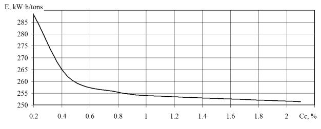
Fig. 4. The effect of increasing the carbon content in the auger material on reducing the growth rate of energy consumption of the dehydration process MSW after its two-week operation and wear (s = 56850 m)
