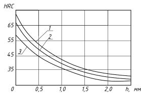
Fig. 3. Changes in the hardness of the depth of the plowshares depending from the recovery method: 1 - restored by welding tires made of steel 45 with sormite surfacing and vibration hardening, 2 - new plowshares made of L-53 steel subjected to vibration hardening, 3 - new plowshares made of steel 65G, strengthened by vibration deformation
