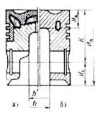
Fig. 3. Piston of forced diesels:a) combined; b) all-metal
