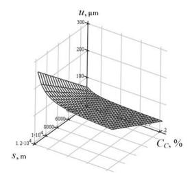
Fig. 3. Dependence of screw wear u in the plane of impact parameters: carbon content in its material  $C_C$  and friction path s
