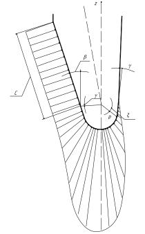
Fig. 1. Scheme of stress distribution in the cutting part of the ploughshare
