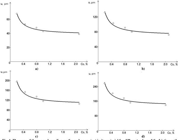
Fig. 1. The wear of the auger depending on the carbon content in its material for different values of the friction path (a) -s = 3000 m, (b) -s = 6000 m, (c) -s = 9000 m, (d) -s = 12000 m: actual  $\circ$ , theoretical —
