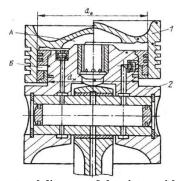
Fig. 10. Structural diagram of the piston with automatic adjusting compression ratio: 1 - piston shell; 2 housing; A and B - respectively, the upper and lower hydraulic cavities
