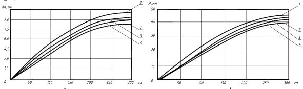
Fig. 5. Changes in wear of width (a) and sock (b) of a plow ploughshare depending on the operating time: 1 - new plowshares made of 65G steel, 2 - restored by welding tires made of steel 45 with sormite surfacing and vibration hardening, 3 - new plowshares made of L-53 steel, subjected to vibration hardening; 4 - new plowshares made of 65G steel, subjected to vibration hardening
