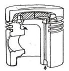
Fig.1. Monometallic pistons of carburetor engines: a) T-shaped; b) U-shaped form
