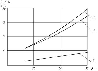
Fig. 2. Curves of changes of efforts on a blade depending on a sharpening angle: 1 - normal component of the cutting force; 2 - component directed along the generative; 3 - total cutting force
