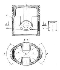
Fig. 12. Combined piston: 1 - piston; 2 - insert
