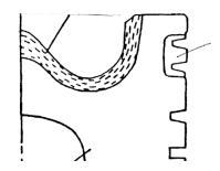
Fig. 11. Combined piston: Al<sub>2</sub>O<sub>3</sub> fibers; niresist; piston (aluminum alloy)
