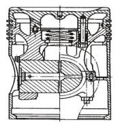
Fig. 8. Composite piston company "MITSUI"
