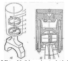
Fig. 5. Piston of the Sulzer engine: a) a sketch of the mechanism of rotation of the piston; b) piston design
