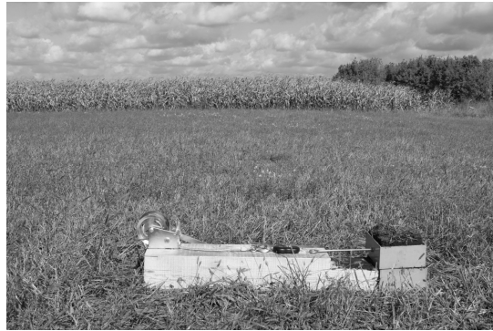
Fig. 3 – Installation for studying the degree of fastening of the abrasive particle in the soil and the coefficient of internal friction of the soil
