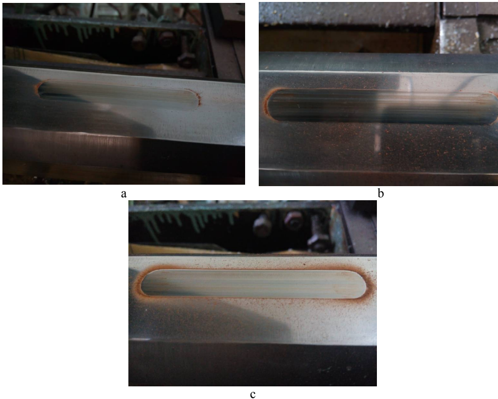
Fig.4. The surfaces of counterbody that worked in the pair with organoplastic based on polychlorotrifluoroethylene reinforced with 20 mass.% of Tanlon fiber at the load: 1,5(a); 2,3(b); 3,2(c) MPa
