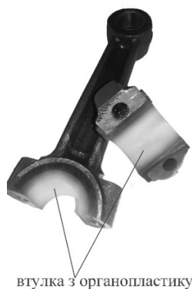
Fig.6. Friction unit of the mechanism of crank mechanism of SO-7B reciprocating compressor
