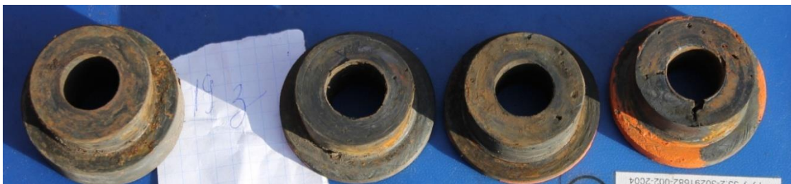
Fig. 9 - General view of experimental details of the upper lever after testing in paralelogram mechanism of cultivator
