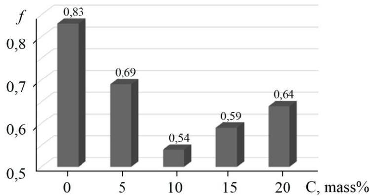
Fig. 1. Influence of carbon fiber on the friction coefficient of polyetheretherketone
