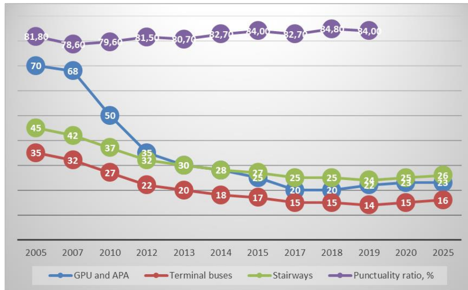
Fig.2. The actual and projected number of certain types of aviation special equipment at the airport, taking into account the introduction of multifunctional PLG
