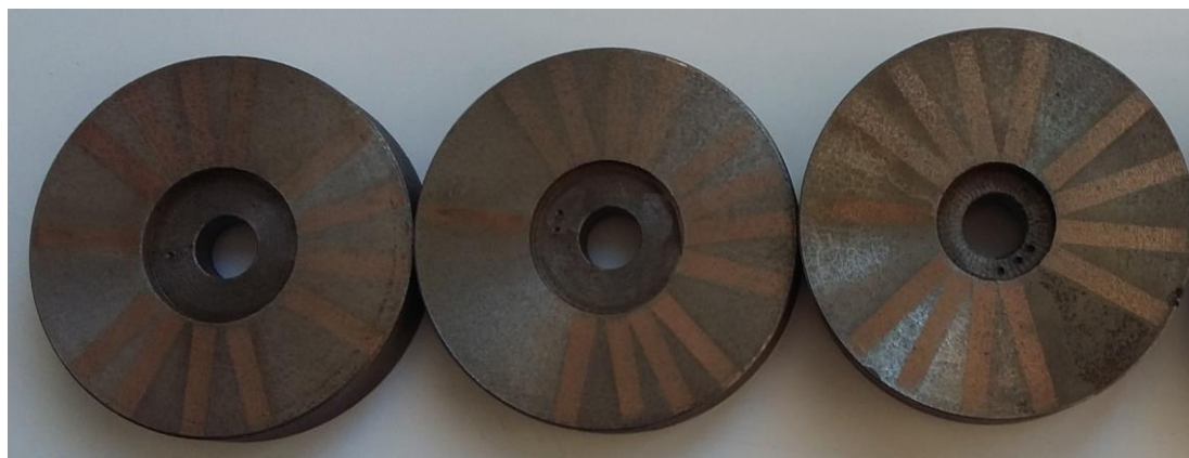
Fig. 4. Studied samples with an antifriction coating applied by a friction-mechanical method
