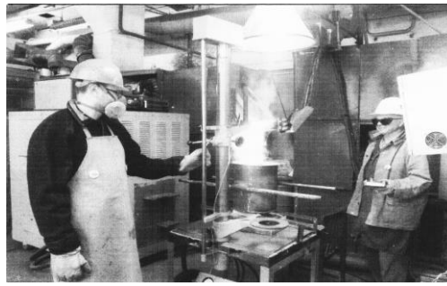
Fig. 3. The process of melting the flux and accumulating slag in the ladle
