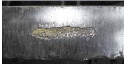
Fig. 2. Exfoliation of the material of the contact element [3]
