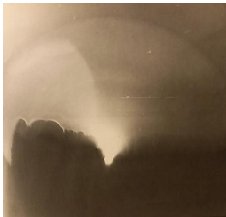
Fig. 3. Electron diffraction pattern from the surface of the contact layer at V=0,5 m/s and P=15 MPa.
