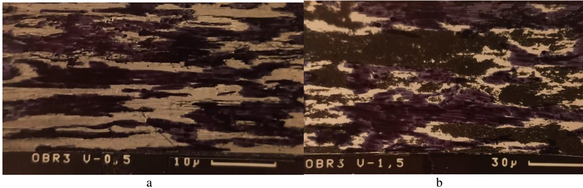
Fig. 2. Topography of friction surfaces coated with a graphite film P = 15 MPa: a - V=0,5 m/s; b - V=1,5 m/s
