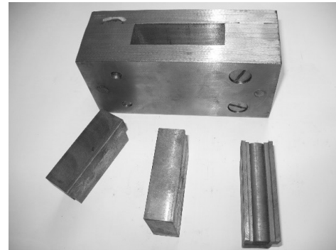
Fig. 5. General view of the mold for graphite inserts
