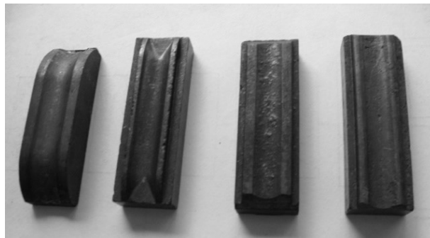
Fig. 2. Types of trolleybus inserts
