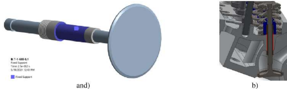
Fig. 6. Attaching the Fixed Support type yokes to the valve guide: a) selected surfaces; b) cross-section of the block head with marking of guide mounting surfaces (red lines)
