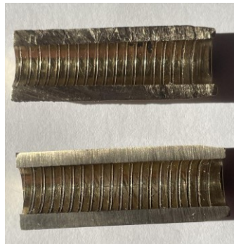
Fig. 5. Spiral oil retaining grooves of the valve guide sleeve
