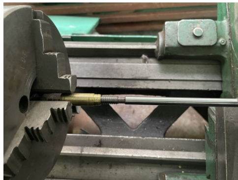
Fig. 4. Treatment of the oil-retaining profile of the valve guide sleeve
