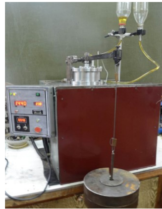
Fig. 4. Scheme of testing a hybrid rolling friction pair [19] - (a); General view of the setup for tribological testing of ceramic balls - (b)
