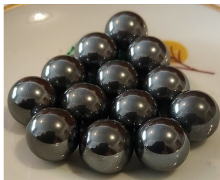
Fig. 3. General view of ceramic balls with a diameter of 12.7 mm after diamond processing
