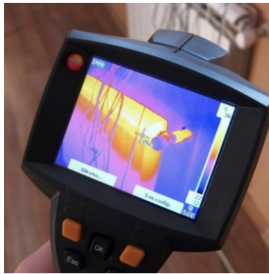
Fig. 4. General view of the portable thermal imager "TESTO-875-2i"
