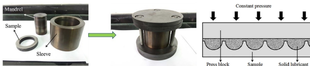
Fig. 9. Experimental tests of solid lubricants for contact strength [28]
