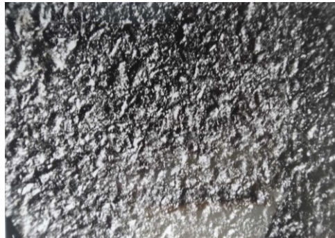
Fig. 11. Surface relief on a forge (steel 45) as a result of the action of an abrasive
