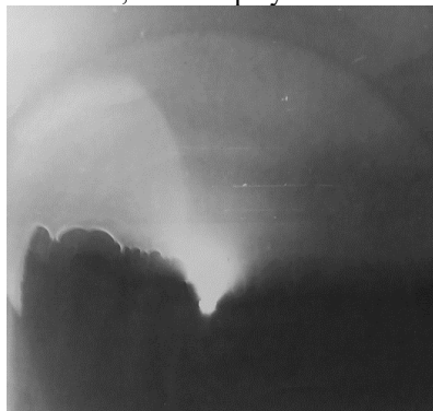
Fig. 4. Electron pattern from the surface of the contact ball orthosilicate-based coating at V=1.5\text{m/s} and P=14.5\text{ MPa} .
