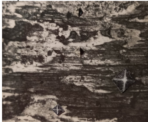
Fig. 5. Surface topography during graphite film formation ( v=0.17 m/s).
