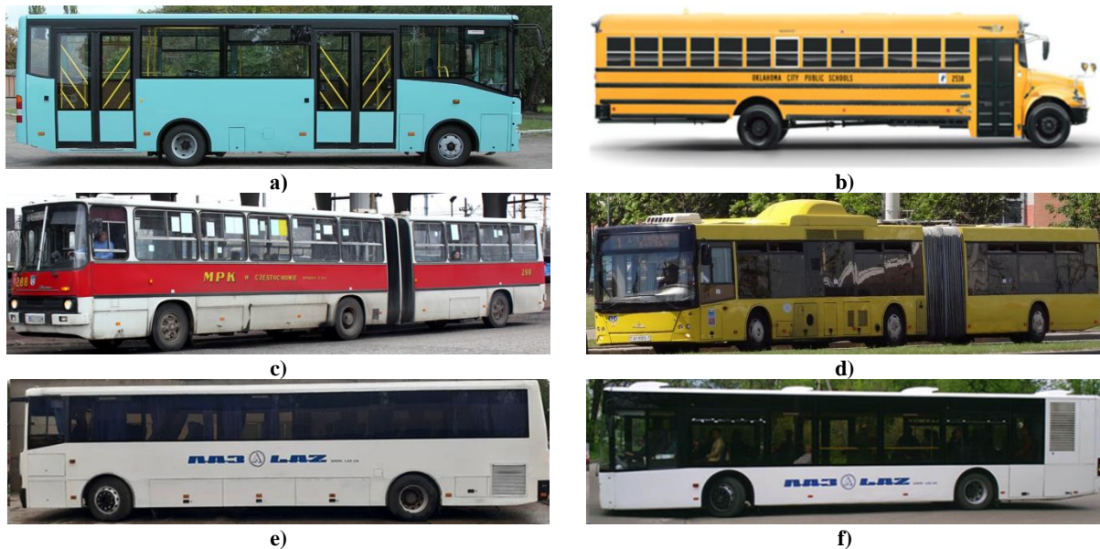
Fig.1 Buses with different engine layouts: a) front with a compartment in the interior; b) front with hood layout; c) middle horizontally under the floor; d) middle vertically; e) horizontally under the rear seats; f) rear vertically with an offset to the left.
