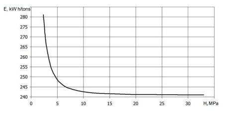
Fig. 2. The influence of the microhardness of the auger coating on the energy intensity of the municipal solid waste dehydration process after its operation and wear on the path s = 56850 m
