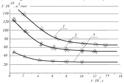
Fig. 6. Dependencies of the change in the volumetric rate of wear during the running-in of tribosystems with different composite materials *RS*<sub>TS</sub>: 1 – steel 40X + steel 40X, (*RS*<sub>TS</sub>=249,9 m<sup>-1</sup>); 2 - steel 40X + VCh 70, (*RS*<sub>TS</sub>=309 m<sup>-1</sup>); 3 - steel 40X + Br.AZH 9-4, (*RS*<sub>TC</sub>=332,5 m<sup>-1</sup>)
