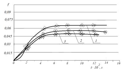
Fig. 5. Dependencies of the change in the friction coefficient during the run-in of tribosystems with different lubricating media  $E_u$ : 1 - hydraulic oil MG–15V ( $E_u$ = 2,43·10<sup>14</sup> J/m<sup>3</sup>); 2 - motor oil M – 10G<sub>2 $\kappa$ </sub> ( $E_u$ = 3,6·10<sup>14</sup> J/m<sup>3</sup>); 3 - transmission oil TSp-15 $\kappa$  ( $E_u$ = 4,18·10<sup>14</sup> J/m<sup>3</sup>)
