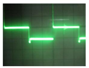
Fig. 3. The shape of the discharge voltage change with a CSD of a rectangular shape with a slit  $\gamma=2$  .
