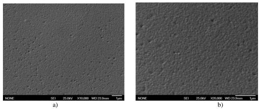
Fig. 3. SEM-images of the Initial Surfaces of the Nanoscaled Detonation Coatings: a) 10 000 zoom; b) 20 000 zoom.
