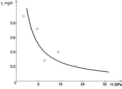
Fig. 1. Dependence of the change in the auger wear rate depending on the microhardness of the coating: actual  $\circ$ , theoretical —
