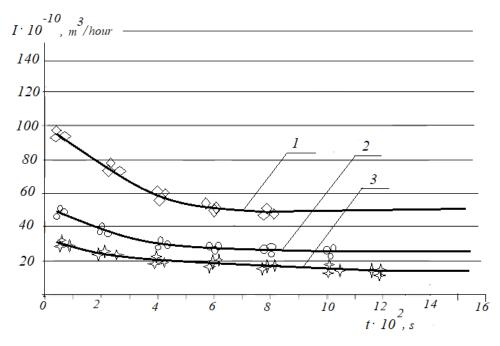
Fig. 2. Dependences of changes in the volume rate of wear during the running-in of tribosystems with different shape factors  $K_{j}$ :  $1 - K_{j} = 5 \text{ m}^{-1}$ ;  $2 - K_{j} = 12,5 \text{ m}^{-1}$ ;  $3 - K_{j} = 20 \text{ m}^{-1}$
