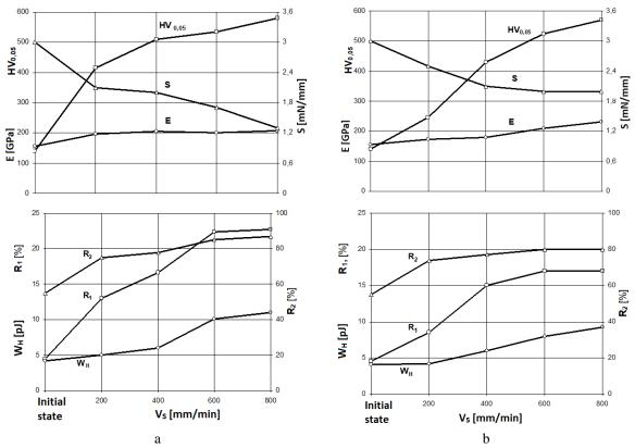
Fig. 7. Effect of arc scanning speed on the micromechanical properties of hardened surfaces at I = 100 A (a) and I = 200 A (b):  $HV_{0,05}$  – microhardness; E – Young's modulus of elasticity; S – contact rigidity; R<sub>1</sub> and R<sub>2</sub> – relaxation capacity in the first and second cycles; W<sub>H</sub> – hysteresis loop area
