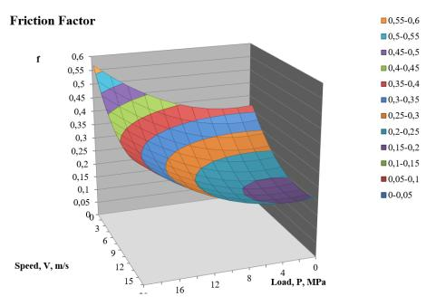
Fig. 2. Diagram of friction factor modeling of nanoscaled coating from friction speed and contact load.
