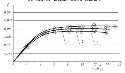
Fig. 7. Dependencies of the change in the friction coefficient during the running-in of tribosystems with different combined materials  $RS_{TS}$ : 1 – steel 40X + steel 40X, ( $RS_{TS}$ =249,9 m<sup>-1</sup>); 2 - steel 40X + VCh 70, ( $RS_{TS}$ =309 m<sup>-1</sup>); 3 - steel 40X + Br.AZH 9-4, ( $RS_{TS}$ =332,5 m<sup>-1</sup>)
