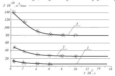
Fig. 12. Dependencies of the change in the volumetric rate of wear during tribosystem running-in for different values of the sliding speed  $v_{sl}$ :  $1 - v_{sl} = 0.2$  m/s;  $2 - v_{sl} = 0.5$  m/s;  $3 - v_{sl} = 0.8$  m/s
