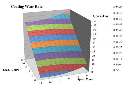
Fig. 1. Diagram of wear rate modeling of nanoscaled coating from friction speed and contact load
