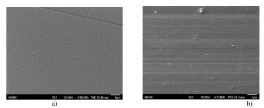
Fig. 5. SEM-images of Sliding Friction Surfaces of the Coatings Developed (10 000 zoom): a) under 0,2 MPa load; b) under 20 MPa load
