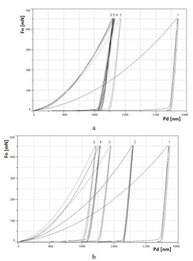
Fig. 6. Kinetic diagrams of continuous indenter microindentation after melting at arc current I = 100 A (a) and I = 200 A (b): 1 - initial state;  $2 - 5 - V_S = 200, 400, 600, 800 \text{ mm/min}$
