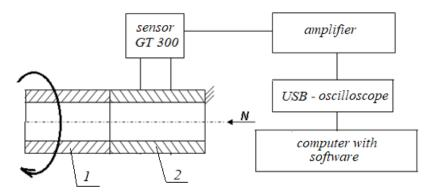
Fig. 1. Block diagram of the experimental equipment for registration and processing of AE signals: 1 - moving triboelement; 2 - fixed triboelement; N - load
