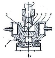
Fig. 2. Four-ball friction machine: 1 - screw; 2 - balls; 3 - friction node; 4 - acoustic probe; 5 - glass; 6 - housing
