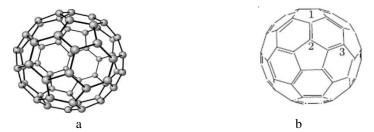
Fig. 1. C60 fullerene molecule: a – general view; в – double bonds between carbon atoms
