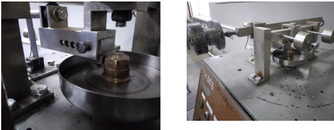
Fig. 1. Schematic representation of the structure of the friction assembly and the tribometer loading mechanism
