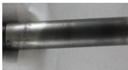
Fig. 7. Pathological wear of the guide part of the intake valve stem from the head side
