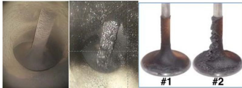
Fig. 5. Deposits on intake valves
