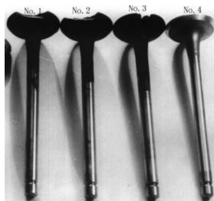
Fig. 2 General appearance of valve damage
