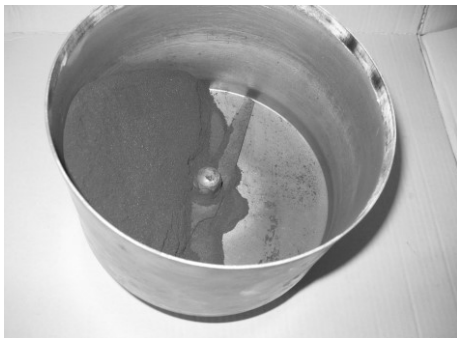
Fig. 4. Crushing of graphite inserts
