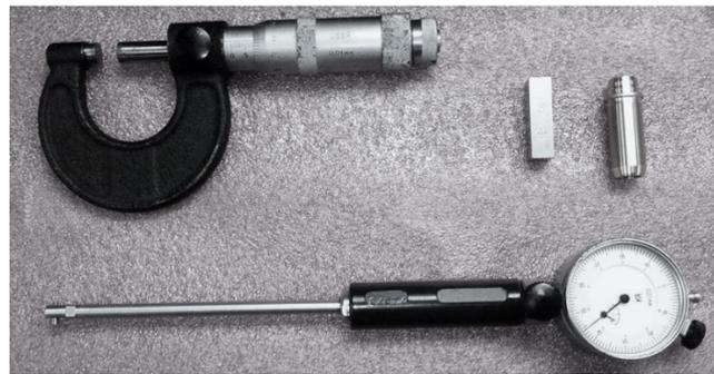
**Fig. 2. Tool for measuring valve bushings.**
