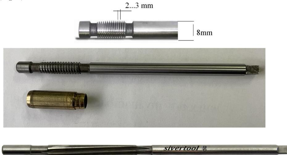
Fig. 3. A special tool for restoring valve bushings.
