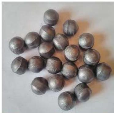
**Fig. 2. General view of sintered ceramic ball blanks**
