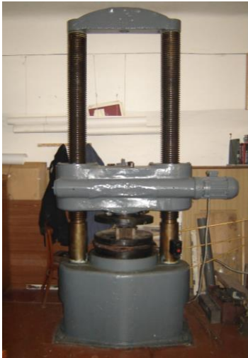
Fig. 1. Hydraulic press PSU-250: Technical characteristics of the press: the maximum admissible loading at compression - 250 ts. ; number of measuring ranges 2; limits of measurement of ranges: the first 25... 100 ts. ; 50... 250 ts. ; the largest stroke of the piston is 50 mm; speed of movement of the working piston -0... 20 mm / min. ; the greatest distance between basic plates is 800 mm; the size of the base plate is 440 x 440 mm.
