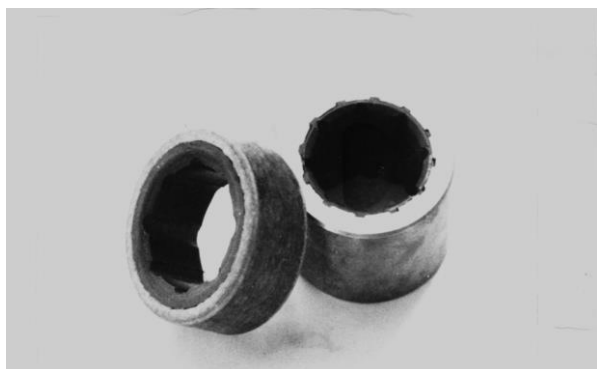
Fig.9 Restoration of the inner diameter of the radial bearing slip
