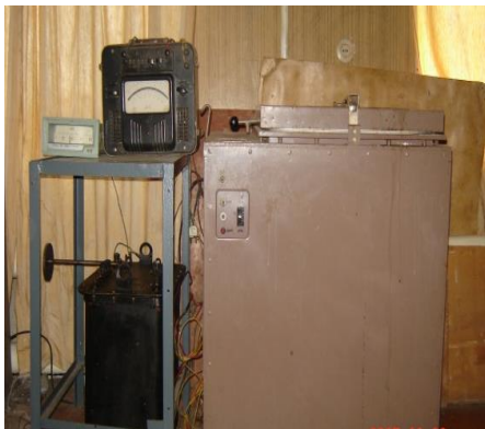
Fig.3 Electric furnace SSHO-3, Technical characteristics: Voltage, at 220; Power, kW- 6; Nominal temperature, ^{\circ}\text{C} - 380
