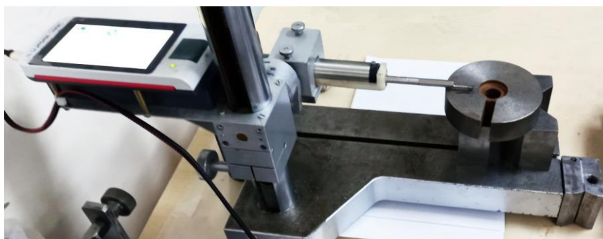
Fig. 3. Weighing a brass tool after FANT (a) and measuring the roughness of the machined surface (b)
