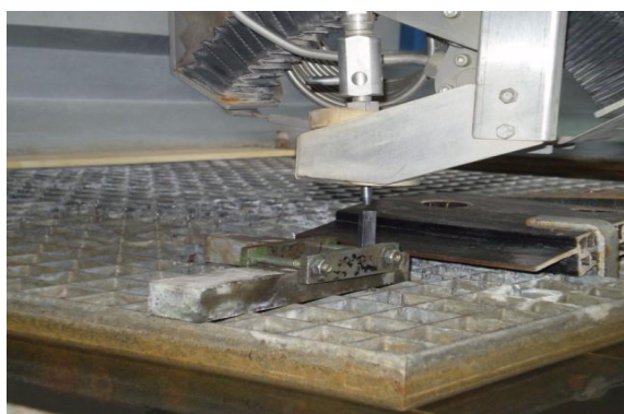
Fig. 8. Installation of a test piece on desktop of hydrocutting machine LSK-5-400
