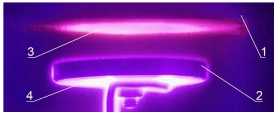
Fig. 2. Burning process of anomalous glow discharge in pulse mode. 1 - anode, 2 - cathode (part), 3 - anode glow, 4 - cathode glow.
